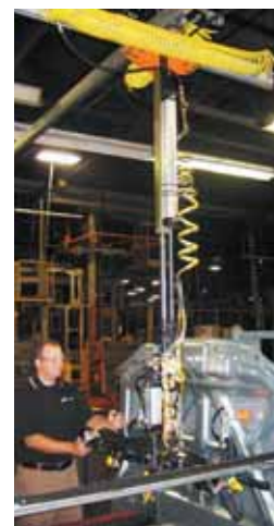
Torque tube with integrated vacuum handling device
