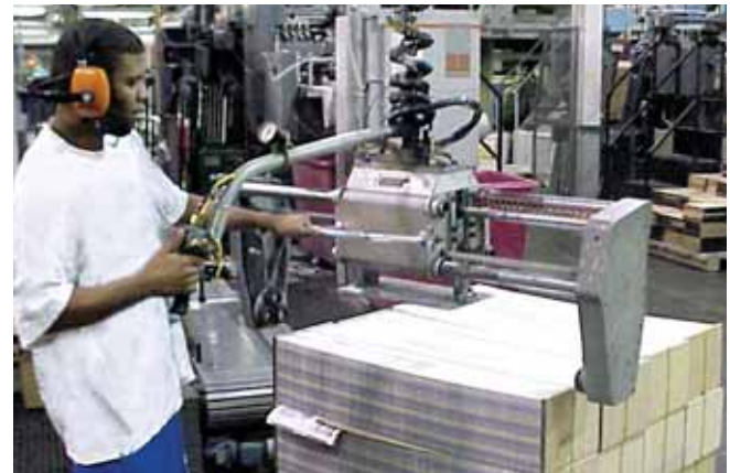
Dual cylinder with top swivel handle control
